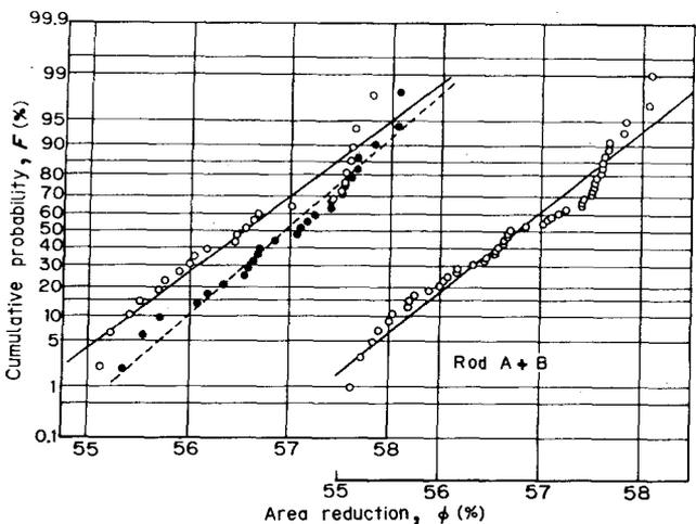
Figure 6 Distributions of area reduction,  $\phi$ . (○) Rod A, (●) Rod B.
