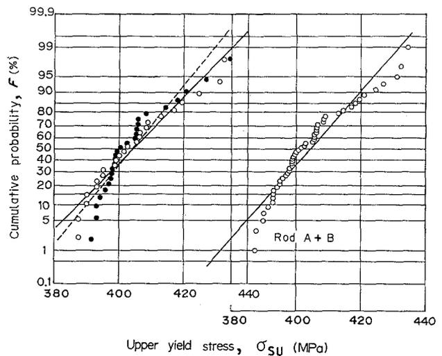
Figure 3 Distributions of upper yield stress,  $\sigma_{SU}$ , (normal probability paper). (○) Rod A, (●) Rod B.
