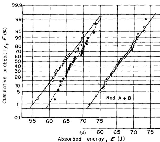
Figure 8 Distributions of absorbed energy,  $E$ . (○) Rod A, (●) Rod B.
