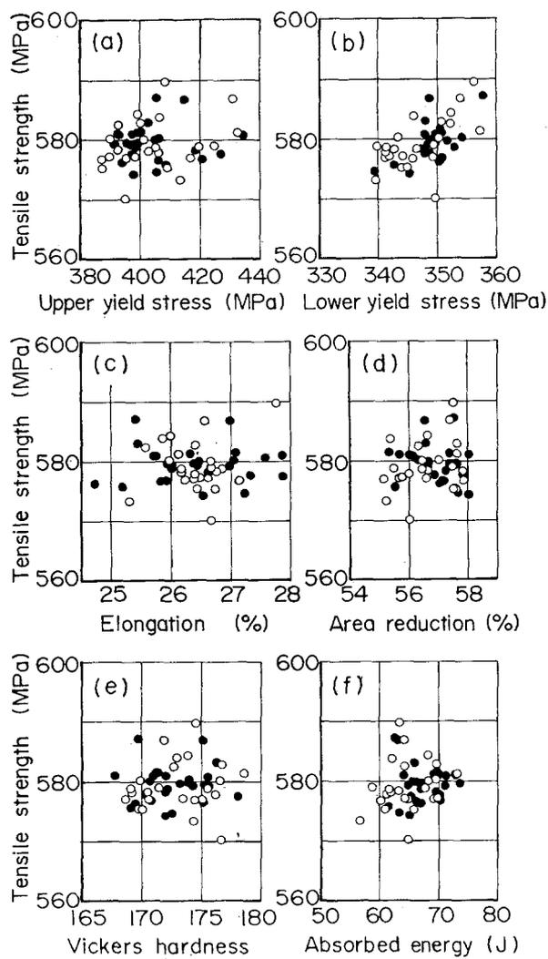
Figure 9 Correlation between tensile strength and other mechanical properties for Rods (○) A and (●) B.
