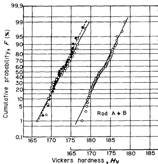
Figure 7 Distributions of Vickers hardness,  $H_v$ . (○) Rod A, (●) Rod B.
