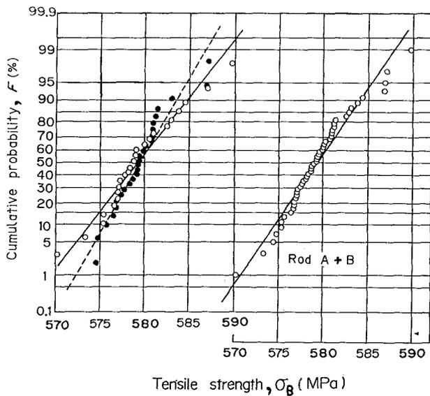
Figure 2 Distributions of tensile strength,  $\sigma_B$ . (○) Rod A, (●) Rod B.
