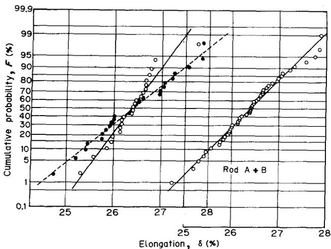
Figure 5 Distributions of elongation,  $\delta$ . (○) Rod A, (●) Rod B.
