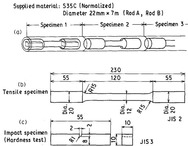
Figure 1 Shapes and dimensions (mm) of specimens.
