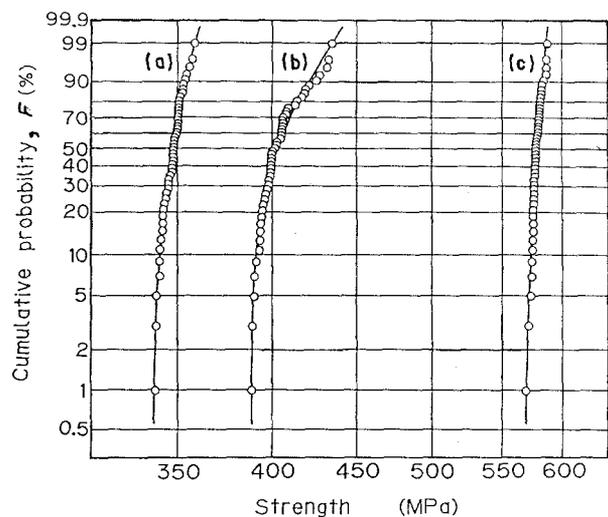
Figure 4. Distributions of (a)  $\sigma_{SL}$ , (b)  $\sigma_{SU}$  and (c)  $\sigma_B$  (Weibull probability paper). (a)  $a = 3.30$ ,  $b = 15.1$ ,  $c = 335$ . (b)  $a = 1.78$ ,  $b = 21.1$ ,  $c = 385$ . (c)  $a = 4.80$ ,  $b = 15.7$ ,  $c = 565$ .
